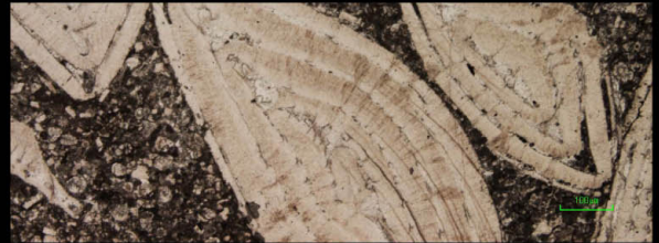
Microscopic view of limestone similar to that used to build Egyptian pyramids. Contains foraminifera, ubiquitous single-celled marine organisms with carbonate shells
